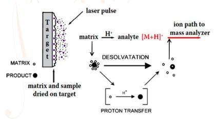
The laser is fired at the matrix crystals in the dried droplet spot placed in vacuum. The matrix absorbs the pulsed (UV) laser energy and get excited. The laser causes desorption of matrix and sample from the microcrystaline surface to vapour phase. The excited matrix molecules adhere proton
