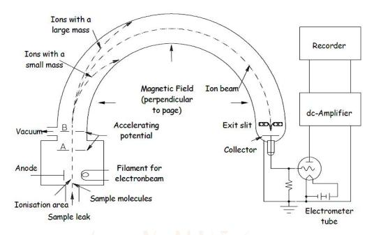
The three essential functions of a mass spectrometer:
