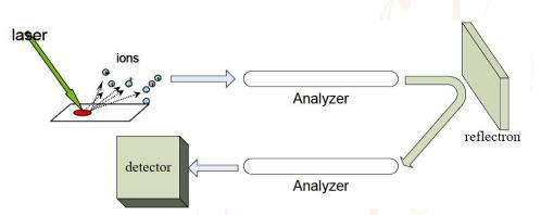
The workflow in reflectron mode is much similar as in linear mode. The only difference is that when the ion hit the reflectron, it will reflect and fly towards the detector. The reflectron focuses ions with the same m/z values, and makes them reach the detector at the same time, which results in more accurate detection.
